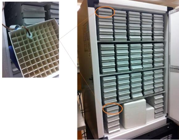
Figure 6: Front top and bottom corner with TC in real sample condition - inside a tube, inside a box.
