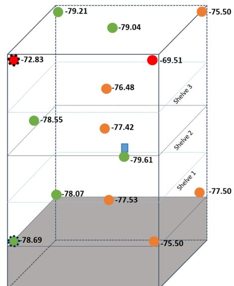
Figure 21: Thermo Temperature Uniformity
