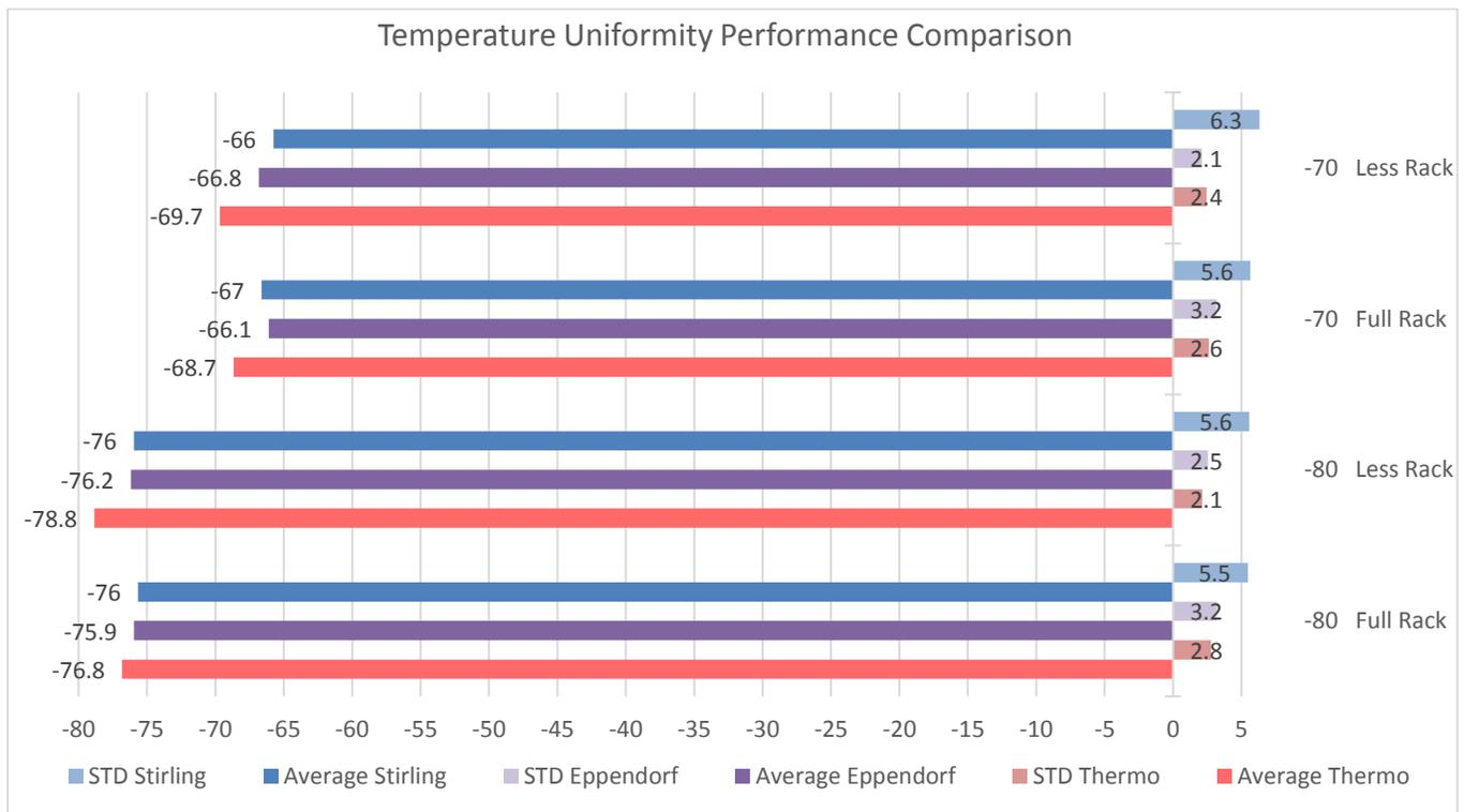
Figure 19: Temperature Uniformity Performance Comparison with standard deviation
