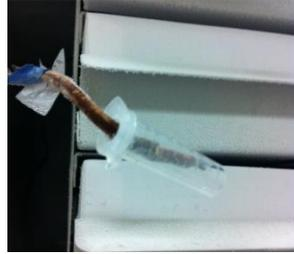
Figure 4: TC inside a plastic tube, inside a box
