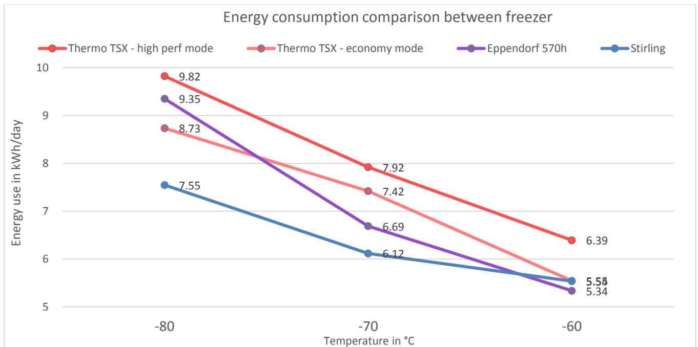
*Figure 9: Energy consumption comparison between freezers*
