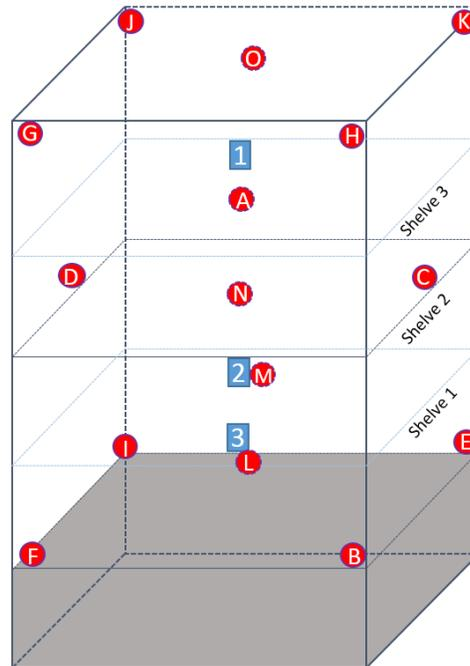
Figure 2: Thermocouple repartition inside the Thermo freezer
