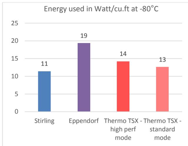
*Figure 10: Energy used in Watt/cu.ft at -80°C*
