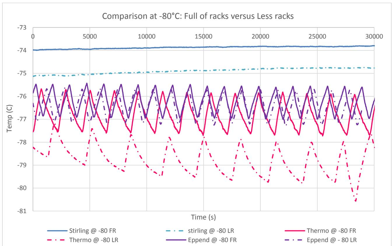
Figure 24: Inside temperature comparison between a unit full of rack and not full of racks
