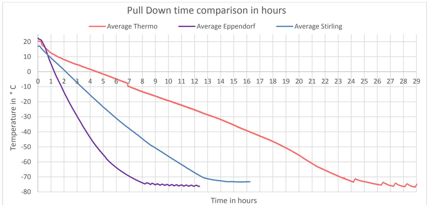
Figure 16: Pull down time in hours
