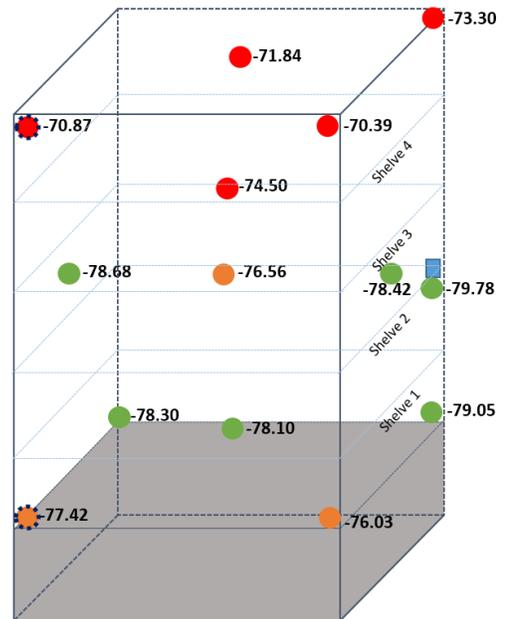
Figure 22: Eppendorf Temperature Uniformity
