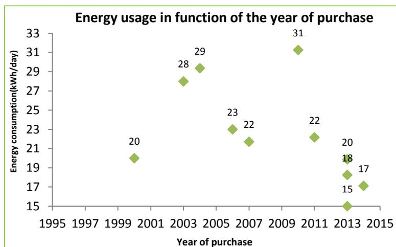
Figure 1: Energy usage of monitored Freezer during the freezer audit in 2014-2015
