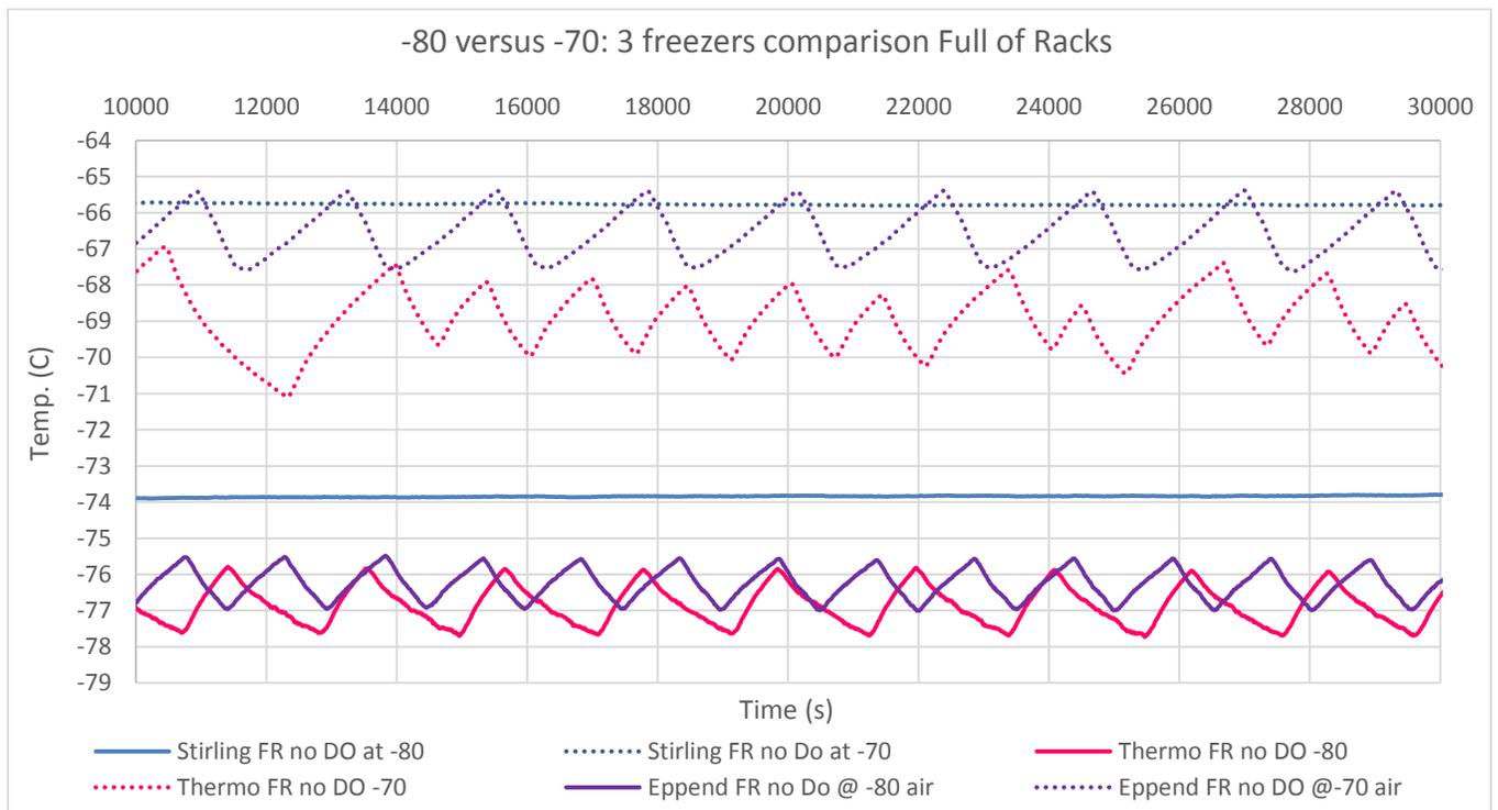
Figure 23: Inside temperature comparison at -70 and -80
