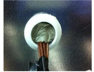
Figure 5: Putty around TCs at the exit of the freezer
