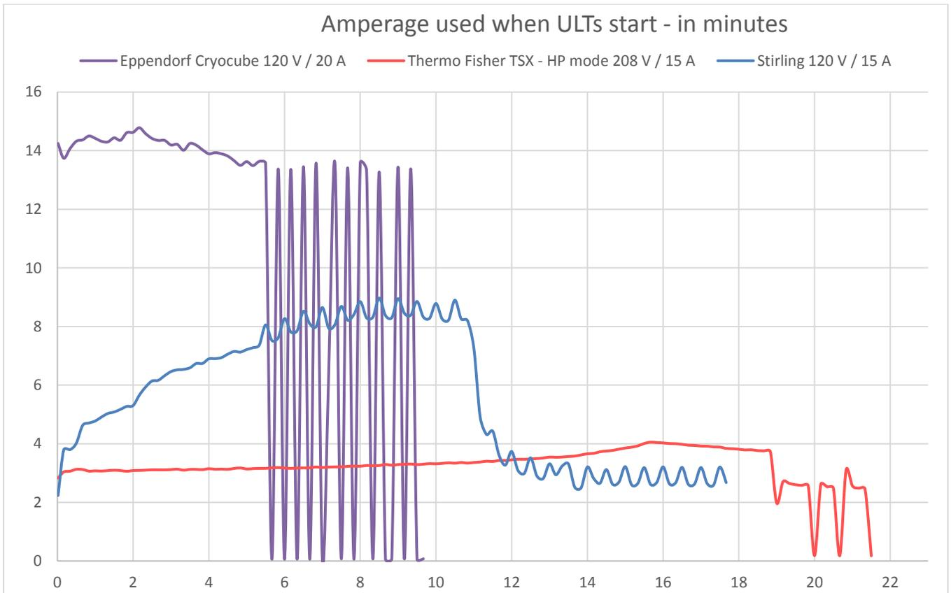
Figure 28: Amperage drawn when the freezers start during the first 20 minutes
