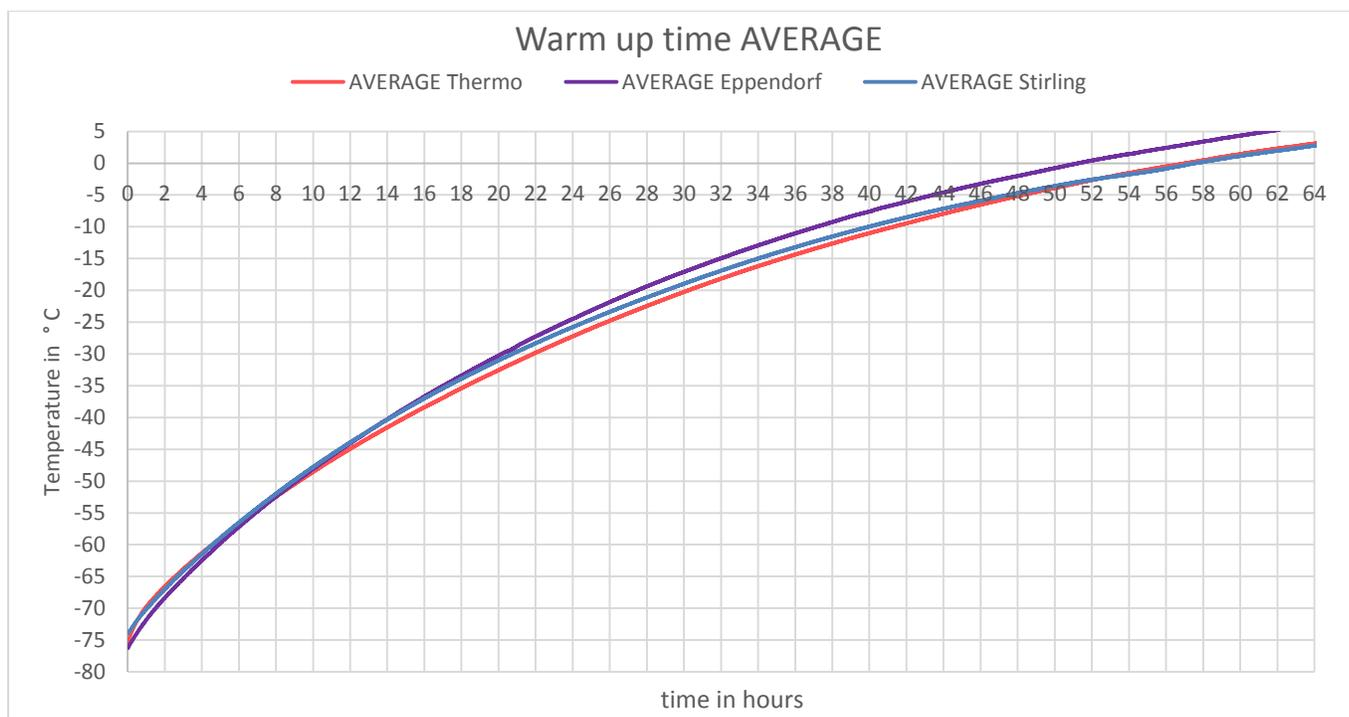
Figure 17: Average Warm up time from -80 to ambient
