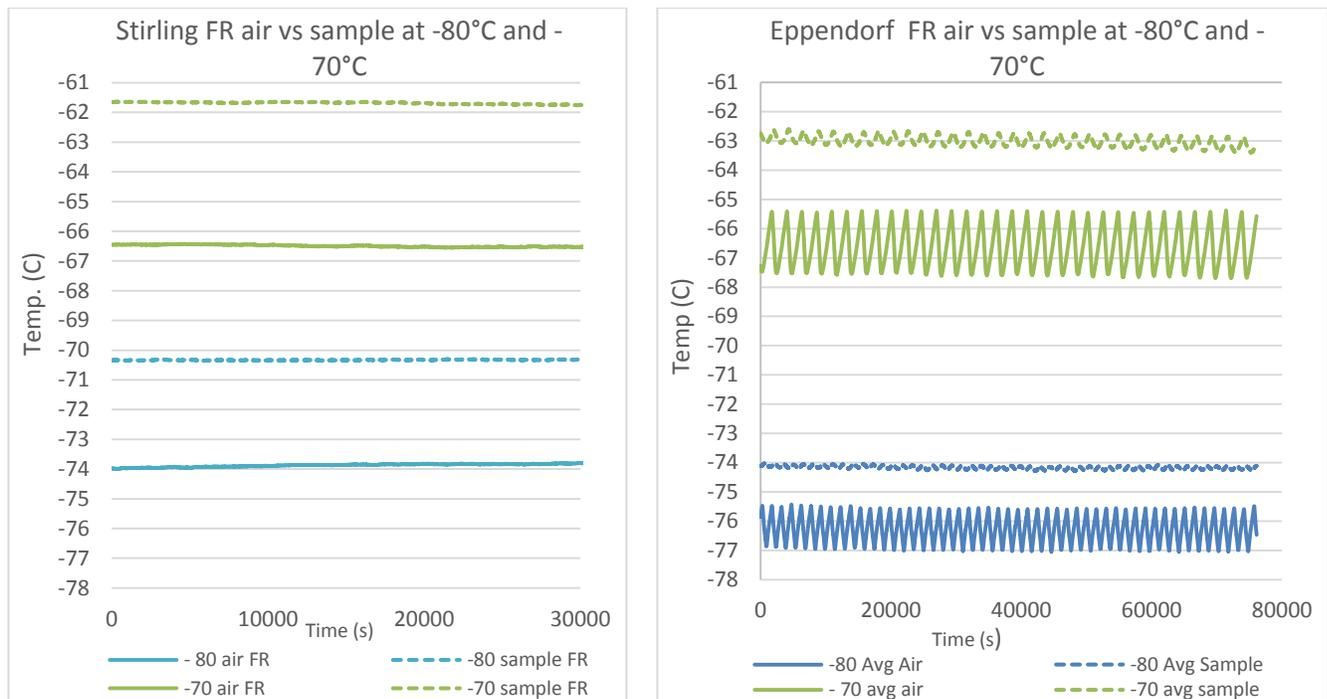
Figure 25: Comparison between air and sample temperature at -70 and -80
