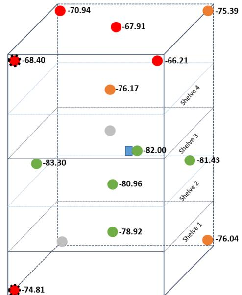
Figure 20: Stirling Temperature Uniformity
